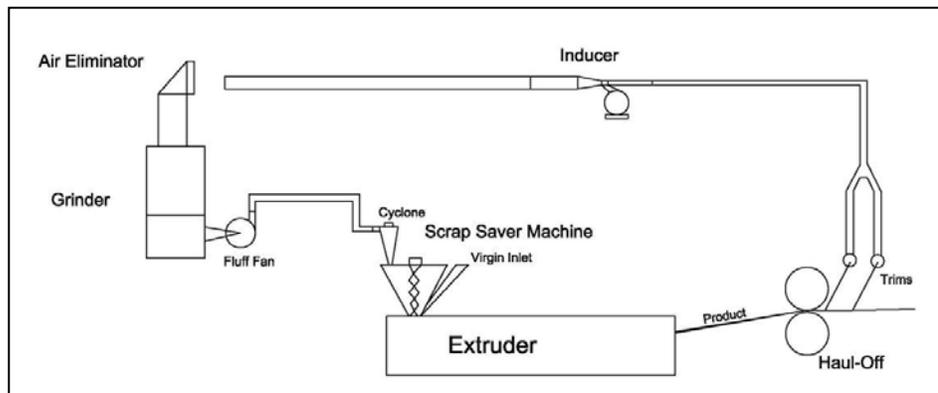
Automatic scrap reclaim system for recovery of trim scrap directly from a winder
