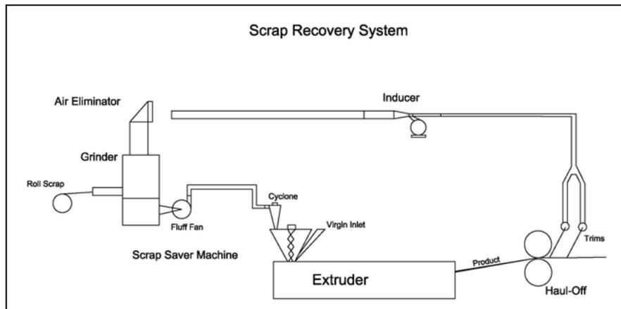
Automatic scrap reclaim system for recovery of trim scrap directly from a winder, and roll scrap from a grinder roll feeder intake.
